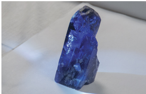
Figure 18. This 765.00 ct tanzanite crystal was heated in an oven at approximately 1000°F to remove all brown coloration. After the temperature was raised incrementally over a number of hours, the peak temperature was maintained for one hour before gradual cooling over a period of six to eight hours. Prior to heating, the crystal was completely brown, with no traces of blue. Photo by Eric Welch.
