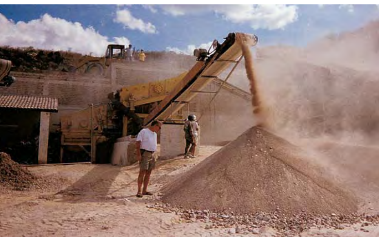
Figure 12. T.O.E. Mineração Ltda. has constructed a large processing plant to recover gem tourmaline from stockpiled mine dumps and alluvial/eluvial material surrounding Morro Alto. Photo by David Sherman.
