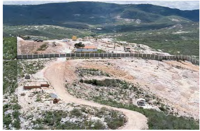
Figure 8. In the early 1990s, numerous near-vertical shafts were dug to explore the pegmatites on Morro Alto at the Mina da Batalha (left). Each shaft is marked by a white dump. A similar view, looking north, is shown in August 2000 (right). Most of the pegmatite dump material and underlying soil have been scraped from the hillside for stockpiling and processing to recover tourmaline fragments. The wall was constructed in the late 1990s to prevent entry into Heitor Barbosa's property. Also visible on the top of Morro Alto in the right photo are a small washing plant (to the left), a new building for the workers, and a water tank. Photos by Brian C. Cook.
