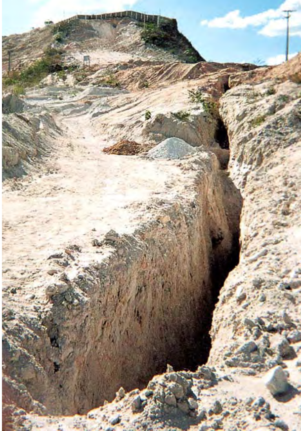
Figure 5. This view, looking northwest in August 2000, shows the excavation of line 6 (called the Jucuri line in this area) that was mined beneath shallow alluvium by T.O.E. Minação Ltda. The narrow width, steep dip, and elongate shape of the dike are typical of pegmatites in the São José da Batalha area. Photo by David Sherman.
