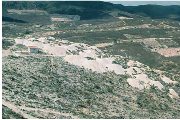
Figure 8. In the early 1990s, numerous near-vertical shafts were dug to explore the pegmatites on Morro Alto at the Mina da Batalha (left). Each shaft is marked by a white dump. A similar view, looking north, is shown in August 2000 (right). Most of the pegmatite dump material and underlying soil have been scraped from the hillside for stockpiling and processing to recover tourmaline fragments. The wall was constructed in the late 1990s to prevent entry into Heitor Barbosa's property. Also visible on the top of Morro Alto in the right photo are a small washing plant (to the left), a new building for the workers, and a water tank. Photos by Brian C. Cook.
