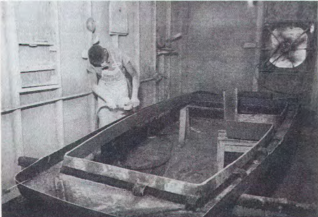
After removal, each component is put through a sanding operation for removal of any rough surfaces.
