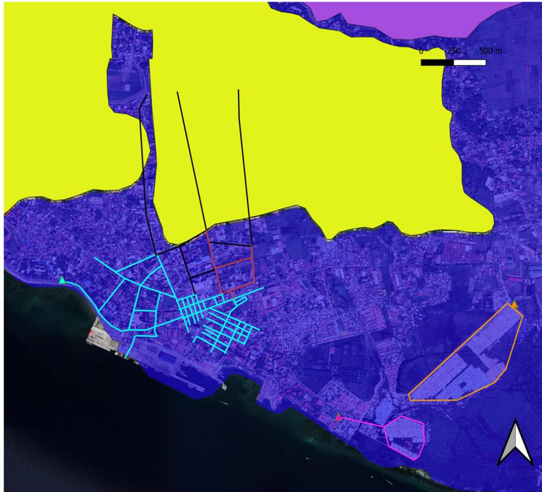
Figure 6-1: Proposed Sewerage Systems in Zamboanga City
